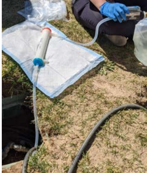
Irrigation water sample collection by dead-end ultrafiltration at a case exposure site in Utah related to an E. coli O157:H7 outbreak. Photo: BreAnne Osborn/Utah Department of Health
