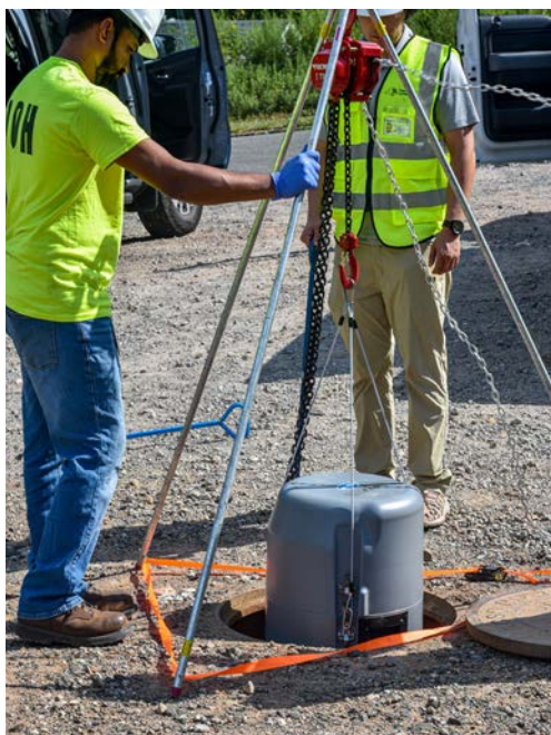
RCDOH and NYSDOH personnel coordinating the deployment of a portable autosampler for upstream sampling in Rockland County in August 2022. Photo: RCDOH
