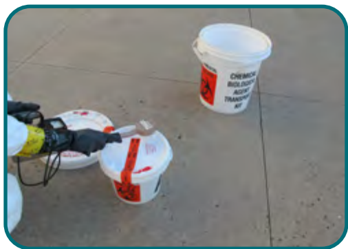
North Dakota Public Health Laboratory staff use a handheld radiation detector to scan over-pack packaging for radiation during a drill to be ready for incidents that may include radioactive material. Photo: ND PHL.
