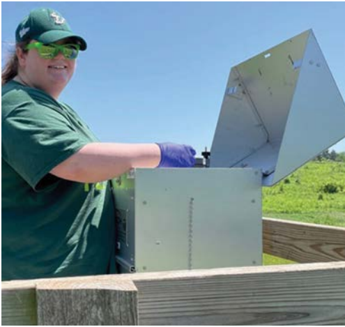
Lexi collects air samples (gas-phase and aerosols) for PFAS analysis using a high-volume air sampler. Photo: Wisconsin State Laboratory of Hygiene
