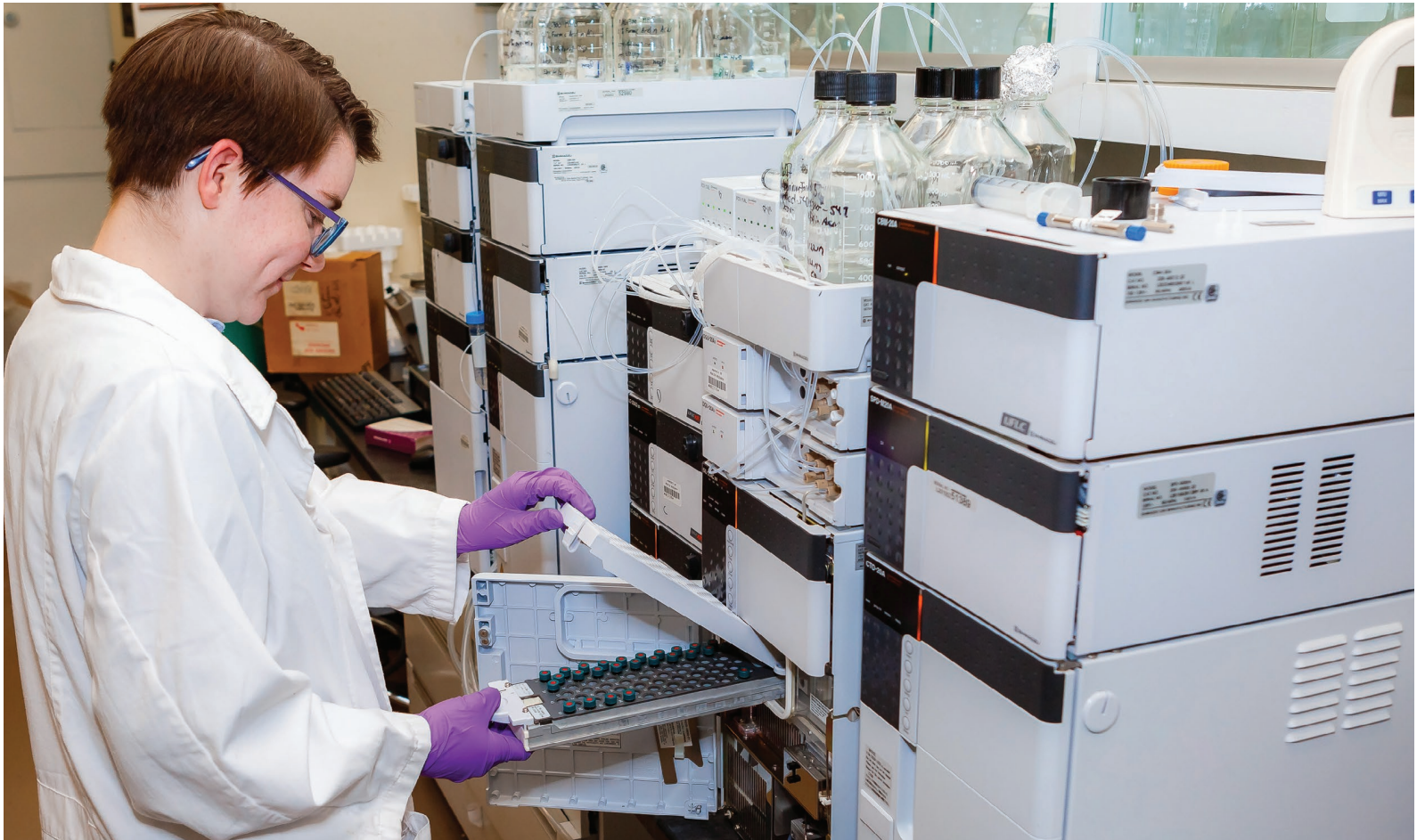
A sample tray of cannabis samples is loaded into the liquid chromatography-mass spectrometer at the Wadsworth Center
